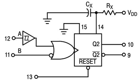
R<sub>X</sub> AND C<sub>X</sub> ARE EXTERNAL COMPONENTS.
