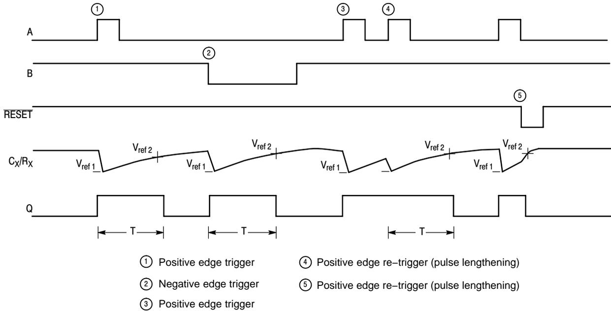
Figure 10. Timing Operation
